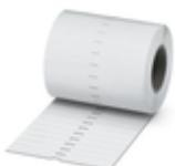
Marking foil for zack marker strip, Roll, white, unlabeled, can be labeled with: THERMOMARK ROLL 2.0, THERMOMARK ROLL, THERMOMARK ROLL X1, THERMOMARK ROLMASTER 300/600, THERMOMARK X1.2, mounting type: adhesive, for terminal block width: 104 mm, lettering field size: 104 x 3.8 mm, Number of individual labels: 2500
